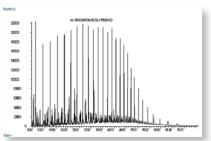
Oil sample chromatogram or "fingerprint" produced by the ERD chemistry team.
